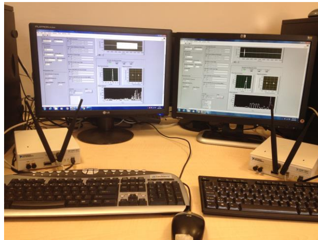
Figure 7. Setup inside WINS Lab. IEEE 802.11b frames are captured using NI USRP and LabVIEW software
